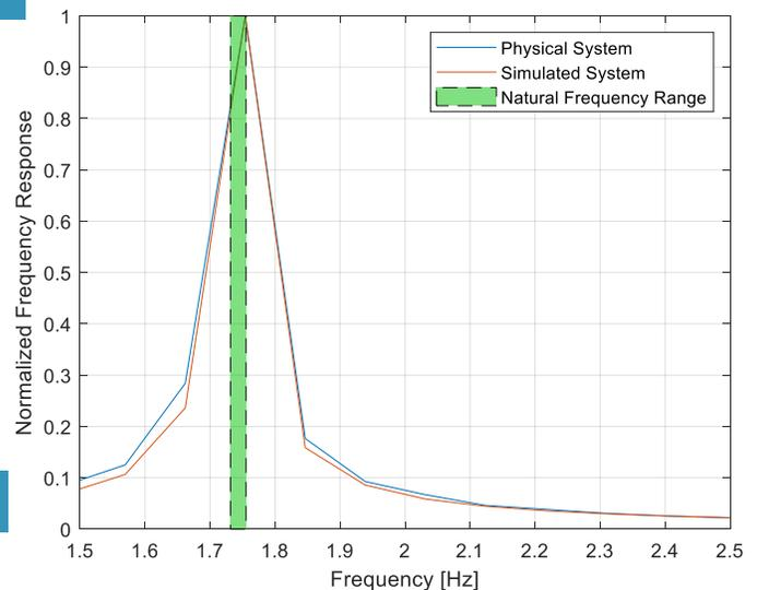
**Figure 6: Frequency Domain Analysis of Physical and Simulated Mass Spring Systems**
