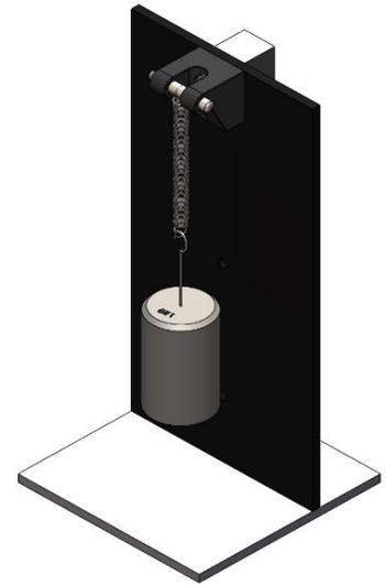
Figure 1: Mass-Spring System CAD Model
