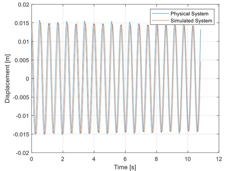
**Figure 5: Time Domain Response of Physical and Simulated Mass Spring Systems**
