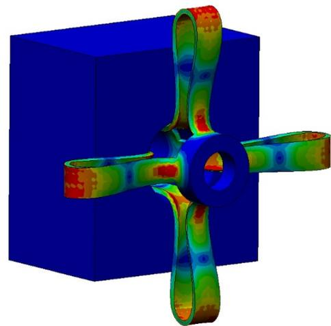
**Figure 1: Static visualization of an FEA result. Stresses are visualized by plotting a colormap over the shape of a deformed part (hot = high stress, cool = low stress!)**
