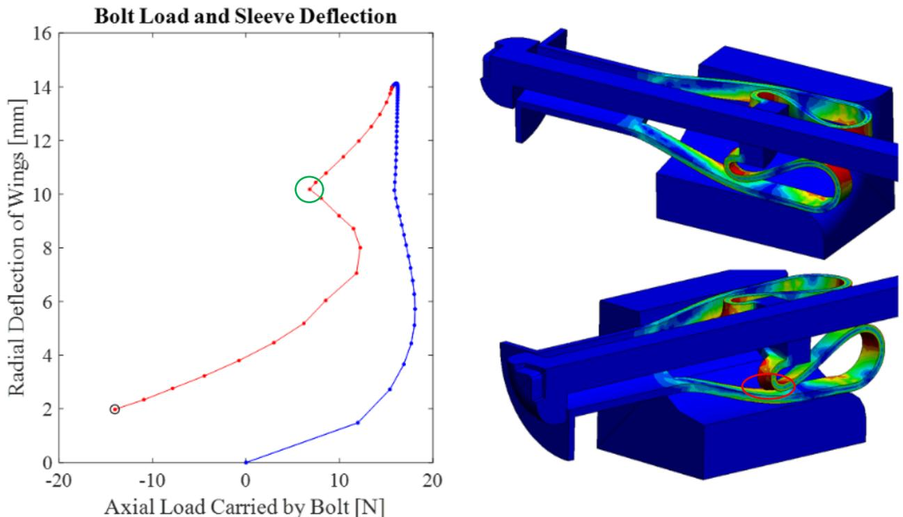
Figure 3 - Still frame from custom visualization. Phase portrait of response variables plotted at left (blue indicates deployment of anchor, red indicates removal; tension is positive, and compression is negative), time-synchronous animation of anchor failure is shown from two angles at right. Visualizations are shown in quarter symmetry, displacements are shown true scale, contour color overlay indicates level of Von Mises
