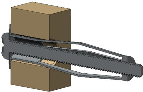
Figure 2 - Drywall anchor before deployment (section view)
